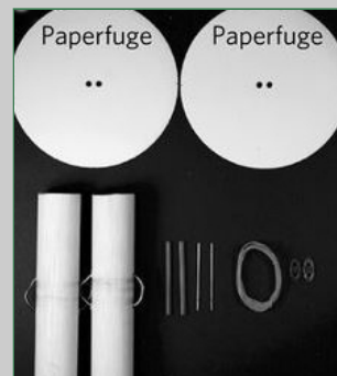
Hand-powered ultralow-cost paper centrifuge , Report on how to make an ultralow-cost (20 cents), lightweight (2 g), human-powered paper centrifuge, called a paperfuge, Nature.com , 17 Aug 2016
